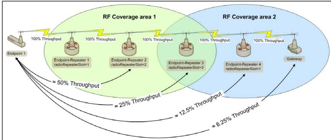
**Figure 233: Multiple Repeaters: Four Endpoint-Repeaters**
