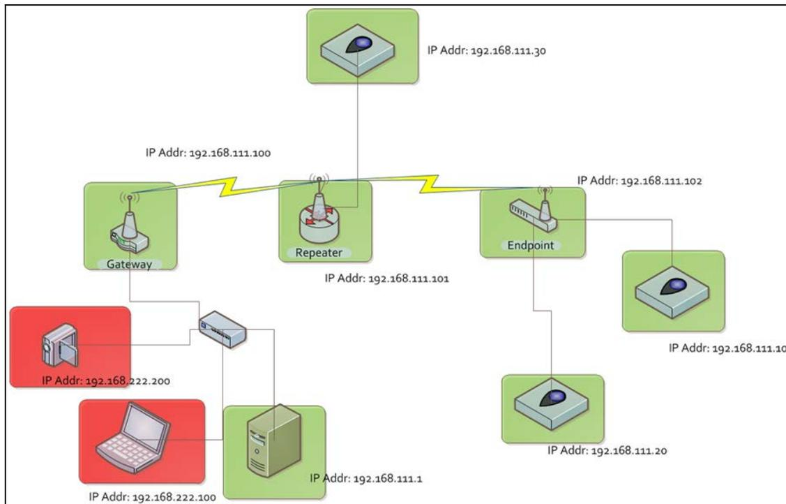
**Figure 223: Network Topology with Traffic at the Gateway but not Desired on the Rest of the Network**
