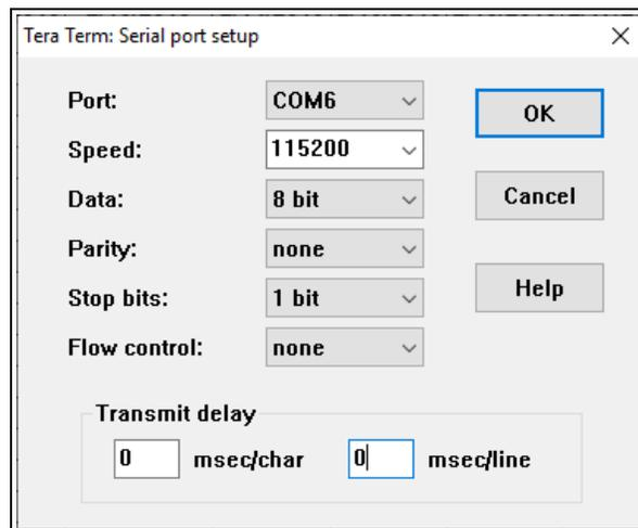
**Figure 220: Tera Term: Serial Port Setup dialog box with Default Settings**
