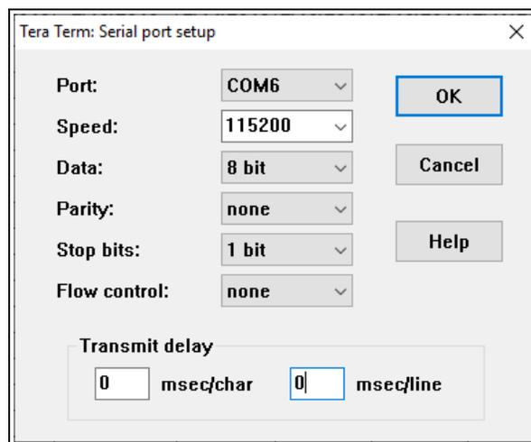
**Figure 227: Tera Term: Serial Port Setup dialog box with Default Settings**
