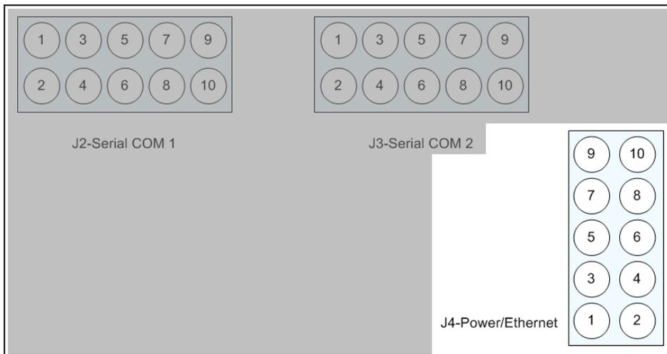
**Figure 3: Z9-PC / Z9-PC-SR001 J4-Power / Ethernet Pinout Assignments**
