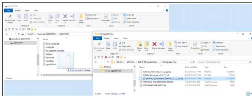
**Figure 74: Drag and Drop the 3\_Optional\_IQ\_Developer\_Edition\_v1\_1\_2\_2.pkg File to the ZumLink window**
