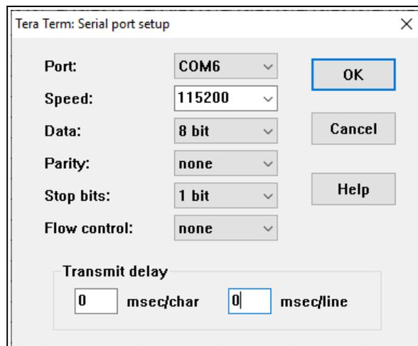
**Figure 56: Tera Term: Serial Port Setup dialog box with Default Settings**
