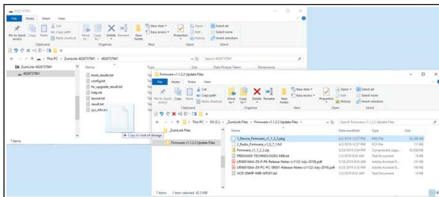
Figure 18: Drag and Drop the **.pkg** file to the **ZumLink** window
