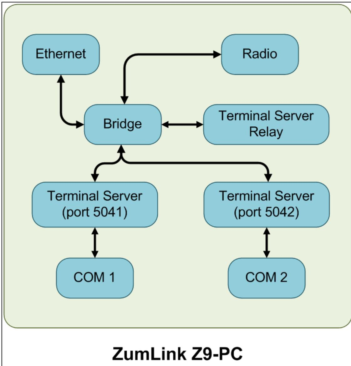
**Figure 236: Terminal Servers and Terminal Server Relay (Client) Connected Together through the Bridge**
