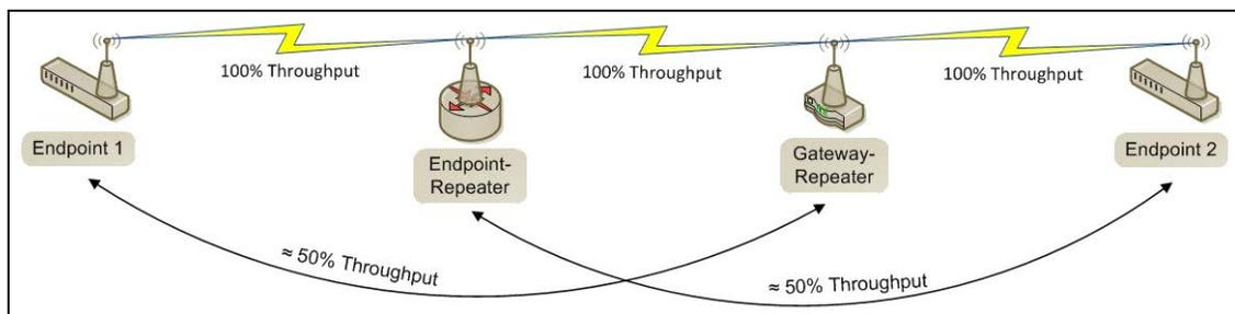
**Figure 232: Repeater with Additional Endpoint to Enhance Connectivity**
