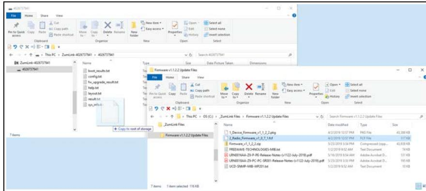
Figure 24: Drag and Drop the **.fcf** file to the **ZumLink** window
