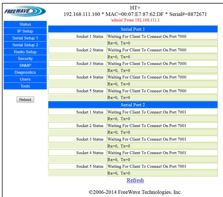
**Figure 31: HTP-900RE and HTP-900SEO Serial Port Status window**
