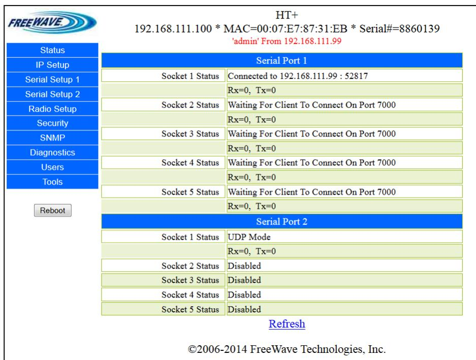
**Figure 58: HTP-900RE and HTP-900SEO Serial Port Status window**
