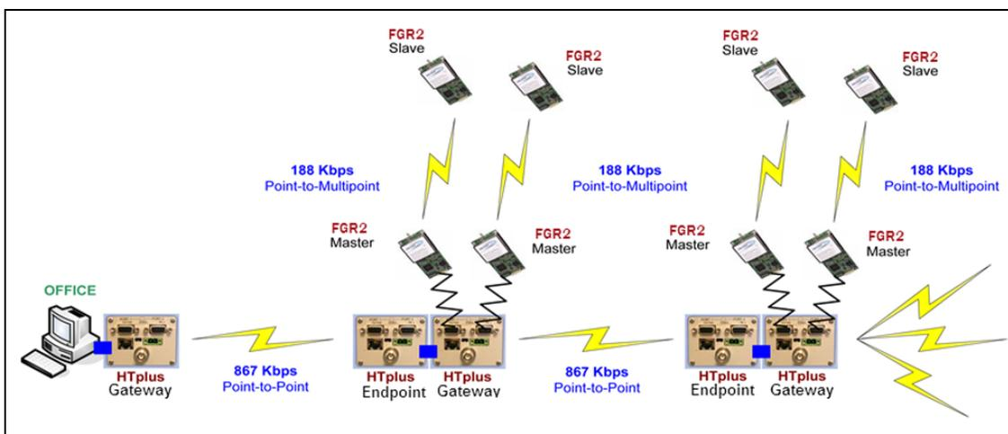
**Figure 32: Example: Configuration of Ethernet and Serial radio connectivity.**
