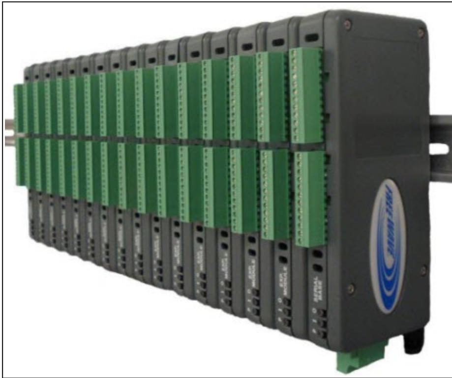
Figure 1: Example of an I/O Expansion stack
