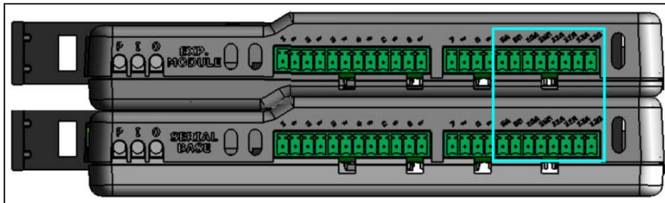
**Figure 17: IO Isolated Channels**
