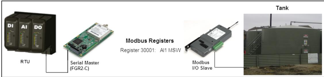
**Figure 16: Example of wire replacement setup to measure tank level.**
