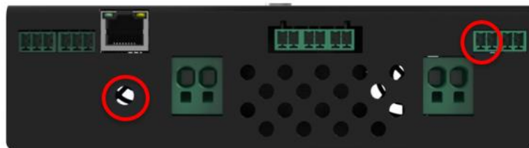
Figure 6 – Temperature sensors (thermal compensation sensors)
