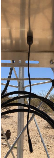
Figure 37 – Correct positioning of the sensor
