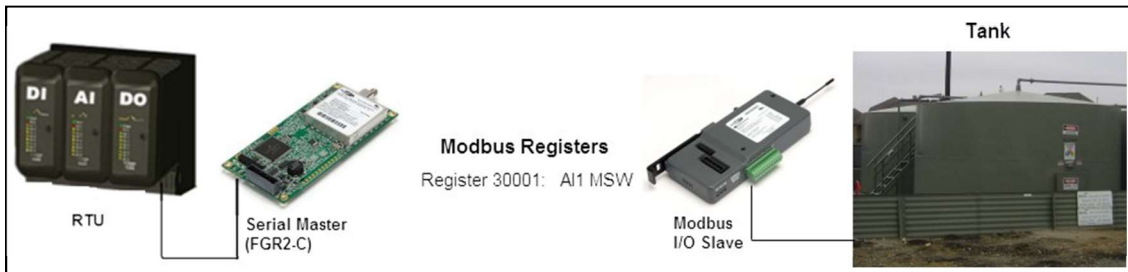
Figure 16: Example of wire replacement setup to measure tank level.
